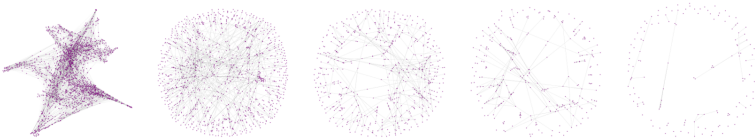
Figure 5: k -NNG graph connectivity layout after each GAT + SAGPool layer, with pooling ratio of 0.5
