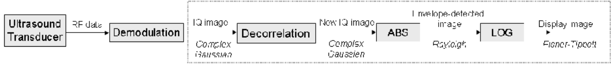
Figure 1. Block diagram. The ultrasound imaging system produces an IQ image, which is the input provided to our approach, which appears within the dotted rectangle.
